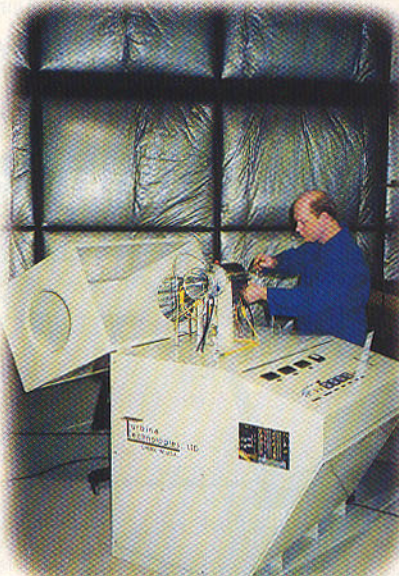
The easy-to-maintain SR-30 engine reaches 87,000 rpm and can be restarted after a 1-minute cool-down.
